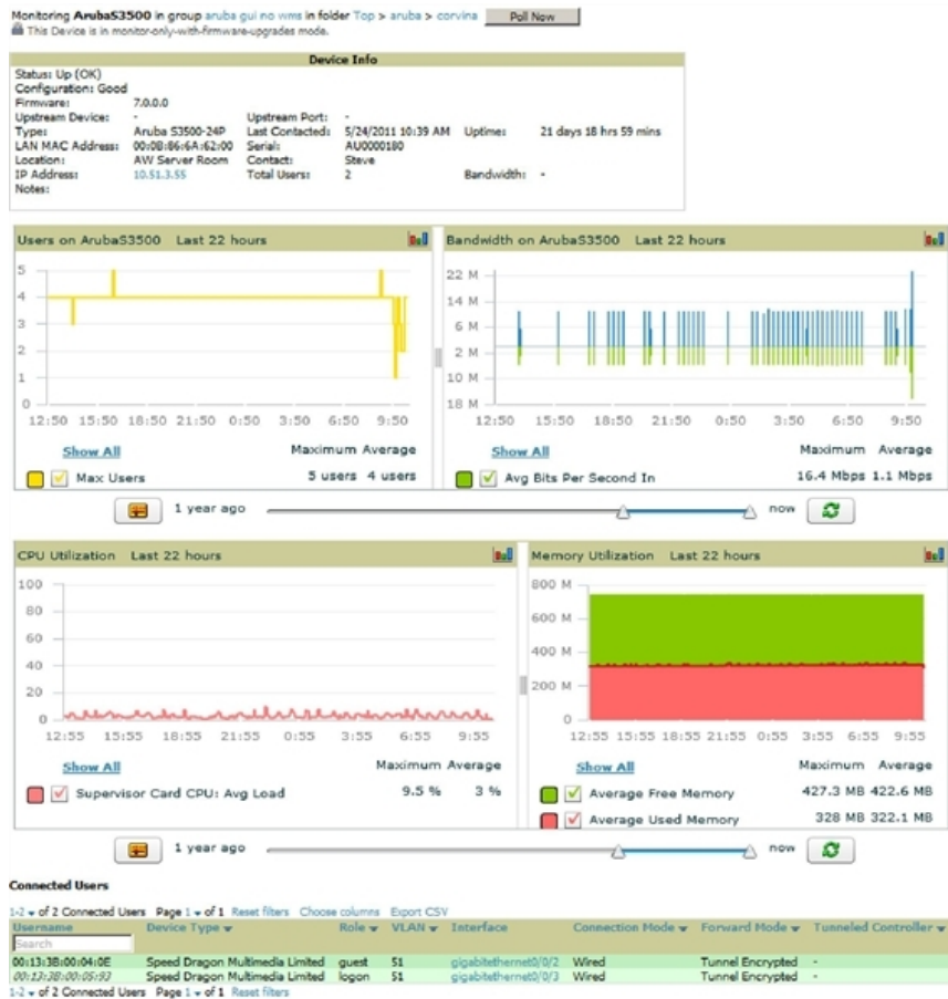
Figure 12: APs/Devices > Monitor Page for a Mobility Access Switch
